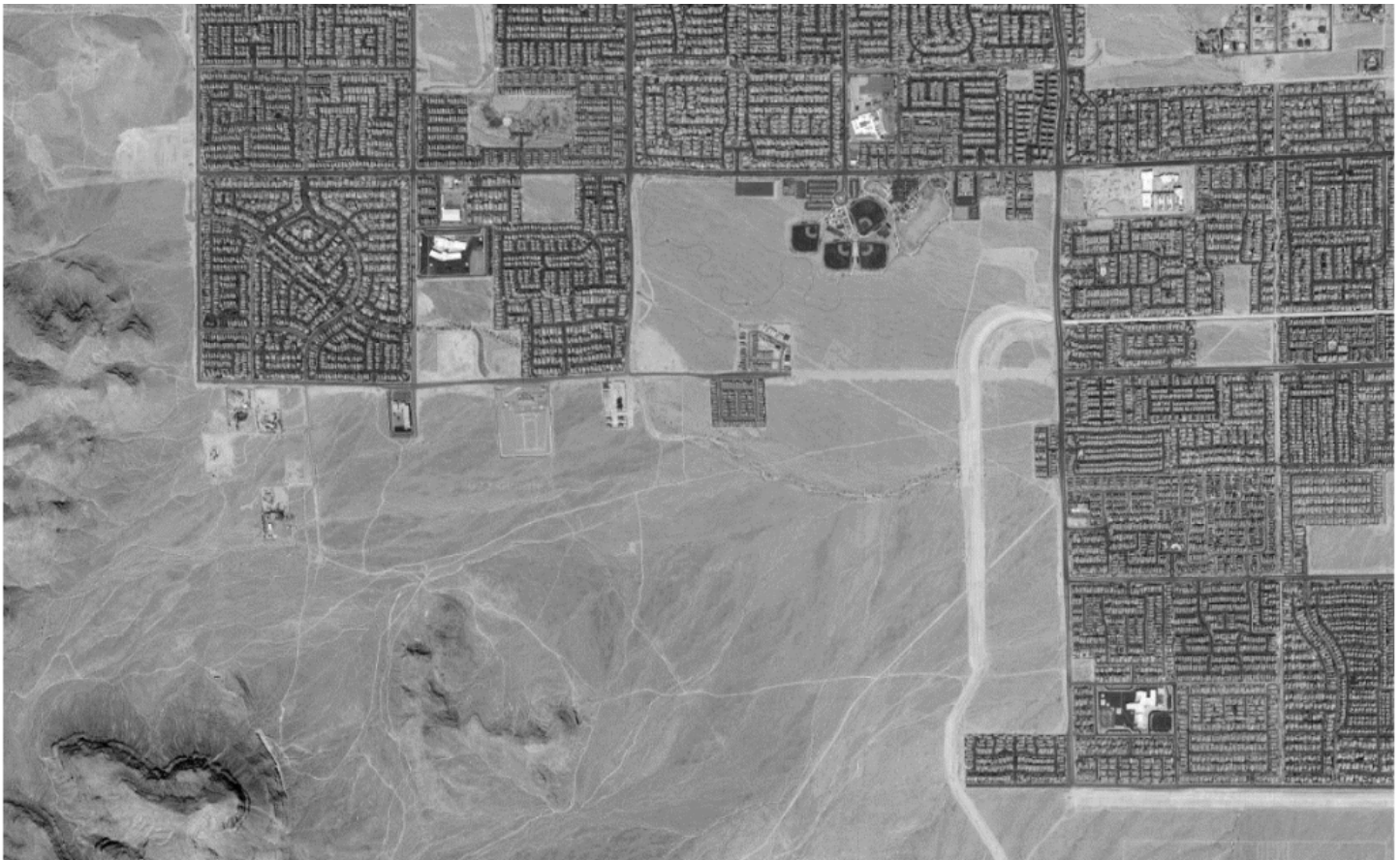
Figure 7 – Satellite greyscale image of southeast Las Vegas and surrounding natural landscapes shows how roofing, wall, and pavement choices in urban environments have relatively low albedos, which influences the quantity of sunlight reflected back to space (Google Maps, retrieved February 19, 2023).
